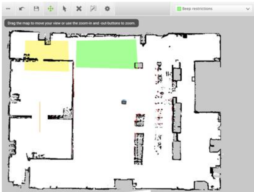
Figure 8.2. Narrow doorways can be marked with a Sound and light zone (marked with yellow) to warn people that it is coming through. A Critical zone (orange) can be placed on the narrow doorway to force the global planner to make a path through the corridor.
